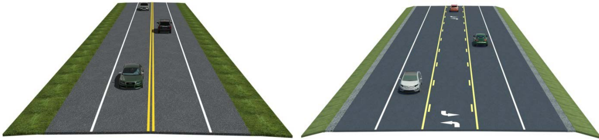
Figure 13 – Two-Lane Typical Sections
